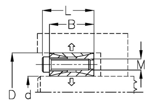
$\begin{array}{lll} \text{B mm} & = 33 \\ \text{d H8 mm} & = 100 \\ \text{D mm} & = 145 \\ \text{Fit tolerance} & = \text{Aksel k11-h11, Nav N11-H11} \\ \text{F kN torque} & = 117.0 \\ \text{L mm} & = 45 \\ \text{M mm} & = \text{M12} \\ \text{P N/mm2 surface pressure on shaft/hub} = 51 \\ \end{array}$
